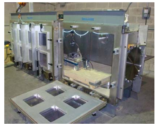
K10mini rover based Regolith Pneumatic Excavator undergoing testing in a 11ft long vacuum chamber.
