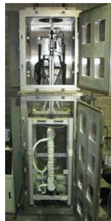
The MoonBreaker drill was tested in the Antarctic lunar analog and vacuum chamber in ice-cemented JSC-1a lunar soil simulant. In both environments, the drill penetrated to 1 meter in 1 hour with 100 Watts and 100 Newton Weight on Bit and acquired samples into a cup.
