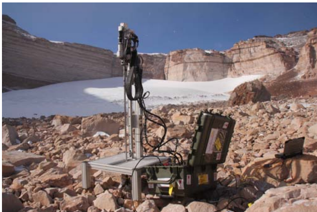
The MoonBreaker drill was tested in the Antarctic lunar analog and vacuum chamber in ice-cemented JSC-1a lunar soil simulant. In both environments, the drill penetrated to 1 meter in 1 hour with 100 Watts and 100 Newton Weight on Bit and acquired samples into a cup.
